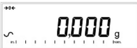
A stable sign  $\sim$  is shown when the unit is in stable condition. It will turn off if the reading is not stable.
