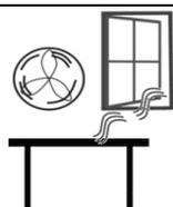
Do not place near open windows, air-conditioning vents or fans that may cause a draft and unstable readings.
