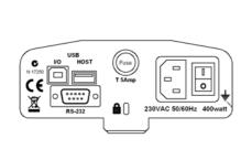
Attach the power supply cable to the connector on the rear of the analyser. The master power switch is on the rear panel, next to the mains cable. Turn the power on.
