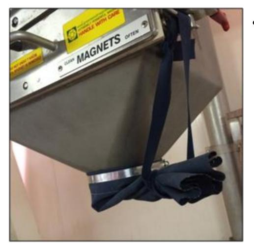
A woven fabric mesh sprayed with a blue neoprene rubber containing ferromagnetic additive.
