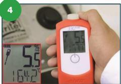
Measurement is complete when TPM% on the display has stopped blinking, and the beacon on the top of the instrument starts flashing (see step 5).
